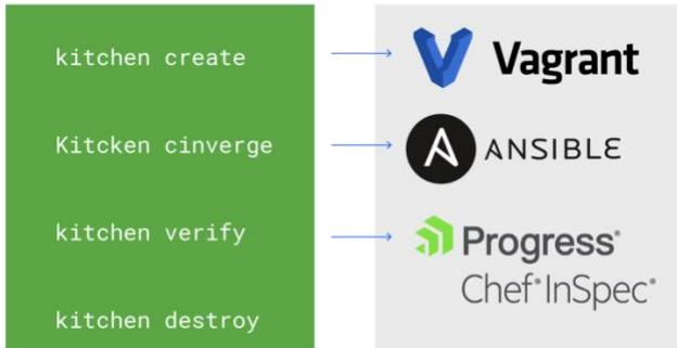
Within Test Kitchen, these steps can be run individually, or all at once via a single command: "kitchen test".
